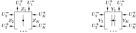
Figure 2: Left: Series K -port scattering junction, with port impedances Z_k , k = 1, \dots, K . Right: Parallel K -port junction, with port admittances Y_k , k = 1, \dots, K .
