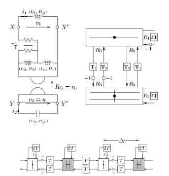
Figure 7: Top left: Transformed MDKC for the (1+1)D transmission line system (21), with  $L_1 = 2\Delta(v_0l - r_0)$ ,  $C_2 = 2\Delta(v_0c - 1/r_0)$ , and  $L_0 = \sqrt{2}\Delta r_0$ . Top right: MDWD network, with  $R_1 = 2L_1/T'$ ,  $R_2 = T'/(2C_2)$  and  $R_0 = r_0$ . Bottom: Expanded signal-flow diagram (port-resistances not shown). Grey/white coloration of junctions indicates calculation at alternating time instants.
