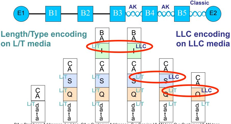
BA = Backbone Addresses, I = I-tag, CA = Customer Addresses, S = Service VLAN tags,Q = Customer VLAN tags.
