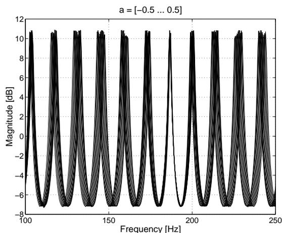
Figure 5: Part of the frequency response of one channel at different  $a_i$  values.
