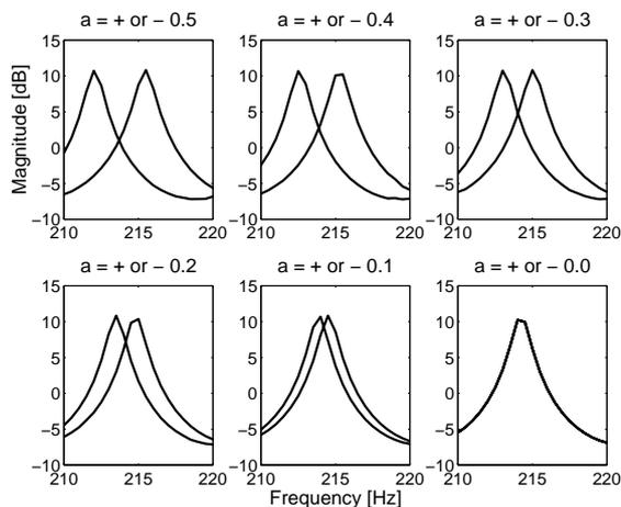
Figure 6: The shift of one frequency peak in one channel at different  $a_i$  values.
