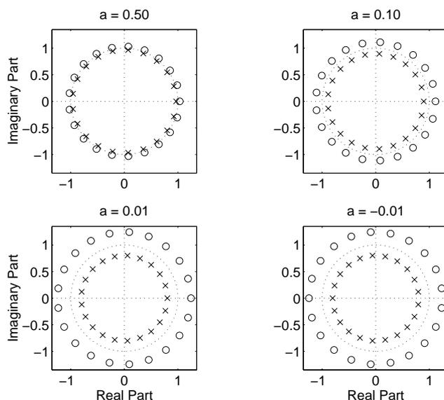
Figure 3: The pole-zero plot of one comb-allpass filter with different  $a_i$  values. The delay  $z^{-D_i}$  inside the filter is 21 samples (defines the number of pole-zeros pairs).
