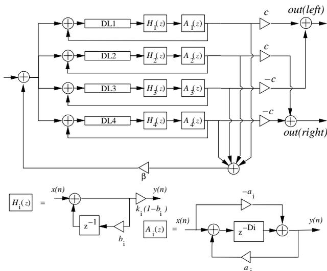
Figure 2: The applied reverberation algorithm, containing four channels [4].
