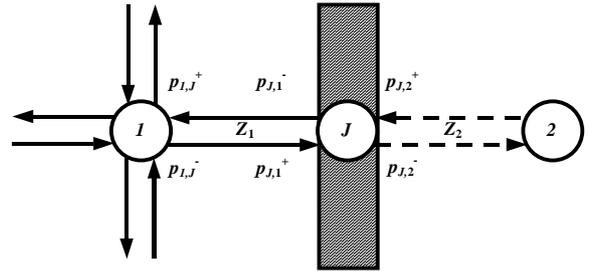
Figure 4: Termination of a waveguide mesh due to a boundary resulting in a reflection.
